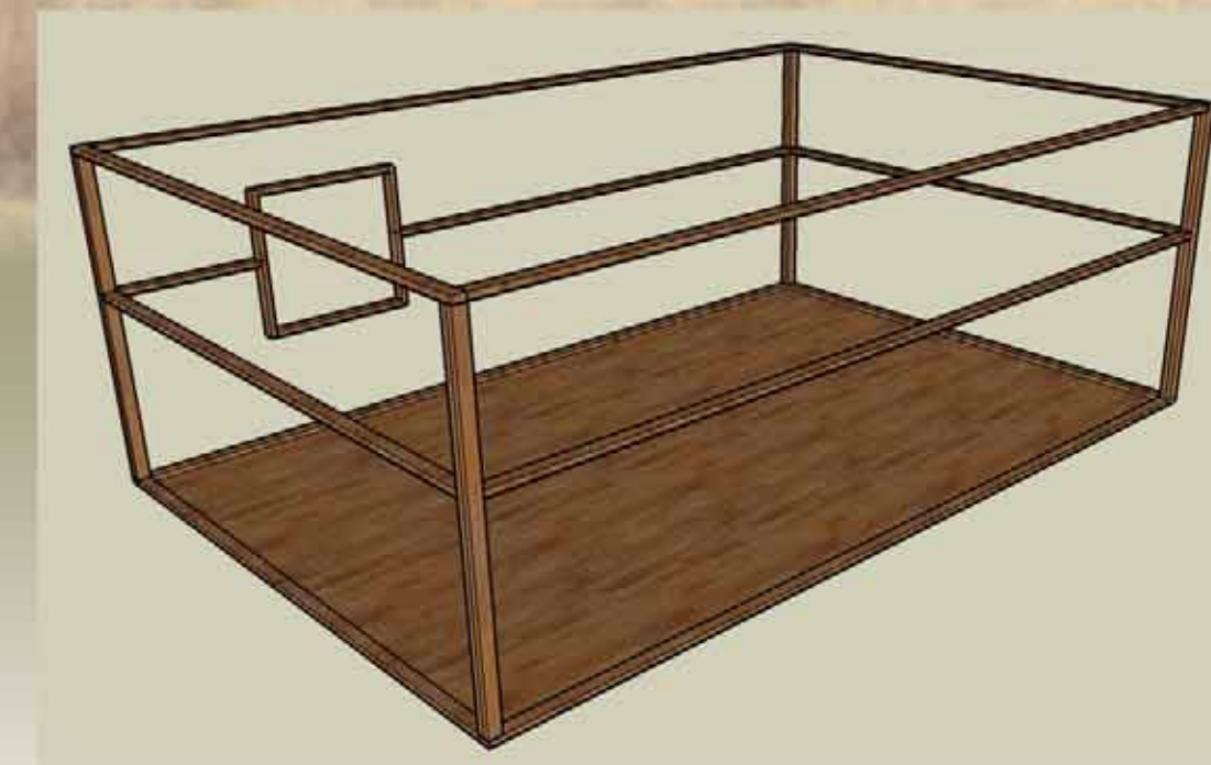
Wood frame of a Straw Bale House
