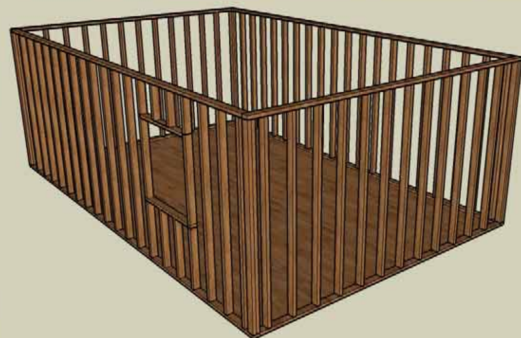
Conventional Wood frame of a House
